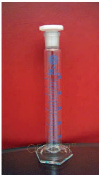
**Measuring Cylinder Round Base** with Interchangeable Polythelene stopper, Class A IAW DIN 12685, ISO 4788 with serially Numbered Individual work Certificate.
