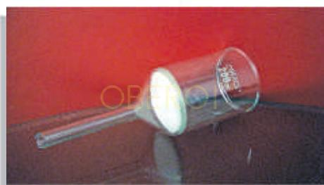
**Buchner Funnel cone at Stem with Sintered Disc porosity Grade G-0 to G-4**
