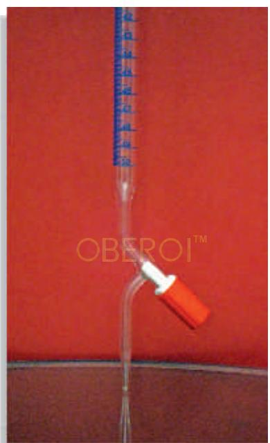
**Burette with Screw type PTFE Stopcock (Needle Valve) Class AS**
