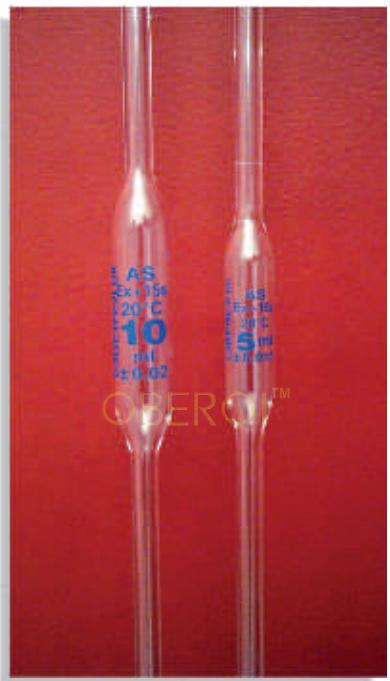
**Pipette Volumetric with one mark. Class AS IAW DIN 12691, ISO 648 with LOT Certificate (waiting time 15 seconds)**
