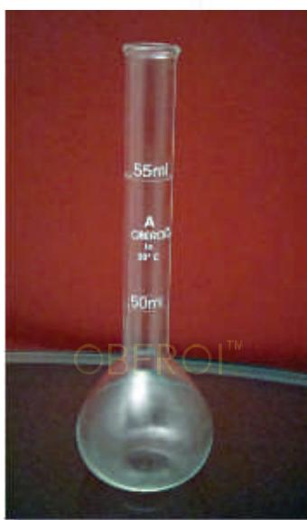
**Volumetric Flask** for sugar Analysis Class A with beaded rim & two marks.
