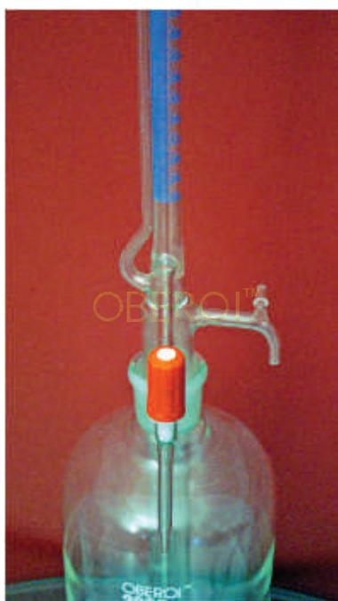
**Burette Automatic Zero** mounted on Reservoir with Screw type PTFE Stopcock (Needle Valve) & Rubber bellow, Class AS IAW DIN 12700
