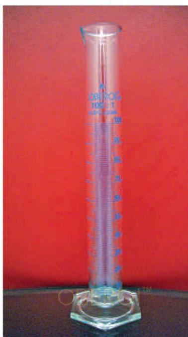
**Measuring Cylinder with spout & Hexagonal Base.** Class A IAW DIN 12680, ISO 4788.
