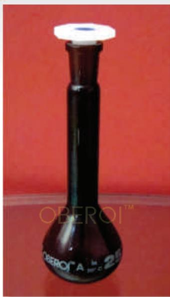
**Volumetric Flask Amber** with one Mark & Polythelene Stopper. Class A IAW ASTM E -228, specification & USP standards. Supplied with Serially numbered Individual work Certificate.
